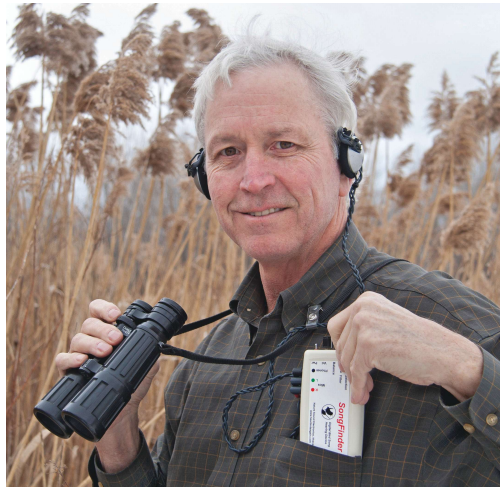
The SongFinder is a pocket-sized device (about 3" x 1" x 5" and 10 ounces) specifically designed for birders who suffer from high-frequency hearing loss. Shown here is Lang Elliott, who invented the SongFinder. Photo courtesy of © Lang Elliott.
