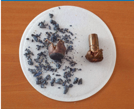
Comparison of two .270-caliber bullets shot into a modified rain barrel for collection to simulate performance on game. The copper jacket lead-core bullet (left) is heavily fragmented compared to the solid copper bullet (right) that retained its original shape upon impact.
