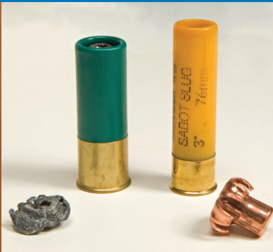
Shotgun slugs made of copper fold into "petals," expanding the slug's surface area better than slugs made of lead.
